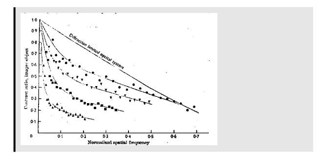
For small pupils (2 mm in diameter) and high spatial frequencies (approaching 50-60 cycles per degree), the human eye is diffraction limited. In other words, no matter how good the optics are, there is a physical limit to the detail that can be resolved--around 60 cycles/degree, the contrast of a 100% contrast grating drops to zero at the retina.
