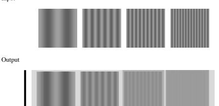
If the input image intensity is  $l(x) = a_f^{\text{in}} \operatorname{Cos}[2 \pi (f x)] + b$ , contrast is defined as  $a_f/b$ .
