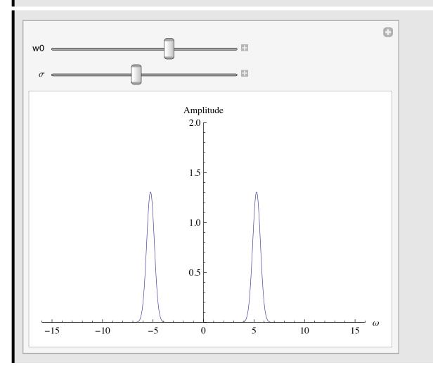
The spectrum is a pair of "blurred out" delta functions, i.e. not as precisely localized in frequency as a pure sinusoid, but nevertheless a gabor function's spectrum is focused around a particular frequency.
