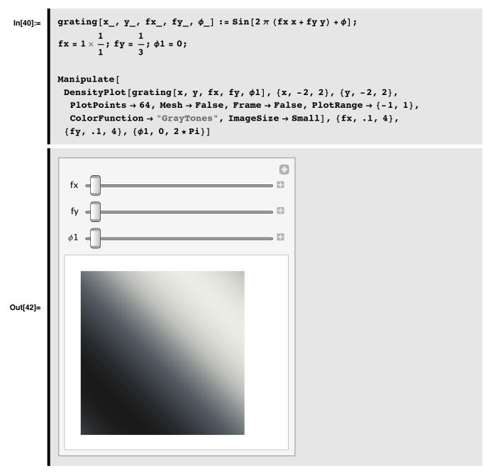
where various combinations of  $\{f_x, f_y, \phi\}$  produce gratings of any spatial frequency, orientation, and phase. Try some variations on the above.
