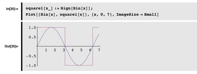
Fourier showed that (almost) any periodic function could be synthesized from a sum of sine and cosine waves. The fourier series for a square-wave is:  $\sum_{n=0}^{\infty} \frac{1}{2n+1} \sin[(2n+1)x]$ . The first term in the series (n=0) is sin(x) and is called the fundamental component of the series. The rest of the components are harmonics. Let's plot up the sum of the first 13 terms together with a plot of the fundamental:
